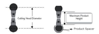
Correct head diameter is required to have proper clearance as the product passes through the cutting head. Having the correct cutting head diameter for your cutoff will result in less speed change or pause and a more constant velocity in cutting head.
