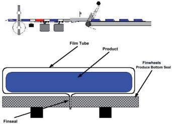
The sealed fin strip is folded over against the package by the auxiliary fin wheels for entry into the endseal jaws. In some cases the machine does not have auxiliary fin wheels. In that case the machine would have a stationary fold over lip to fold the finseal over before entering the Cutting Head area.
